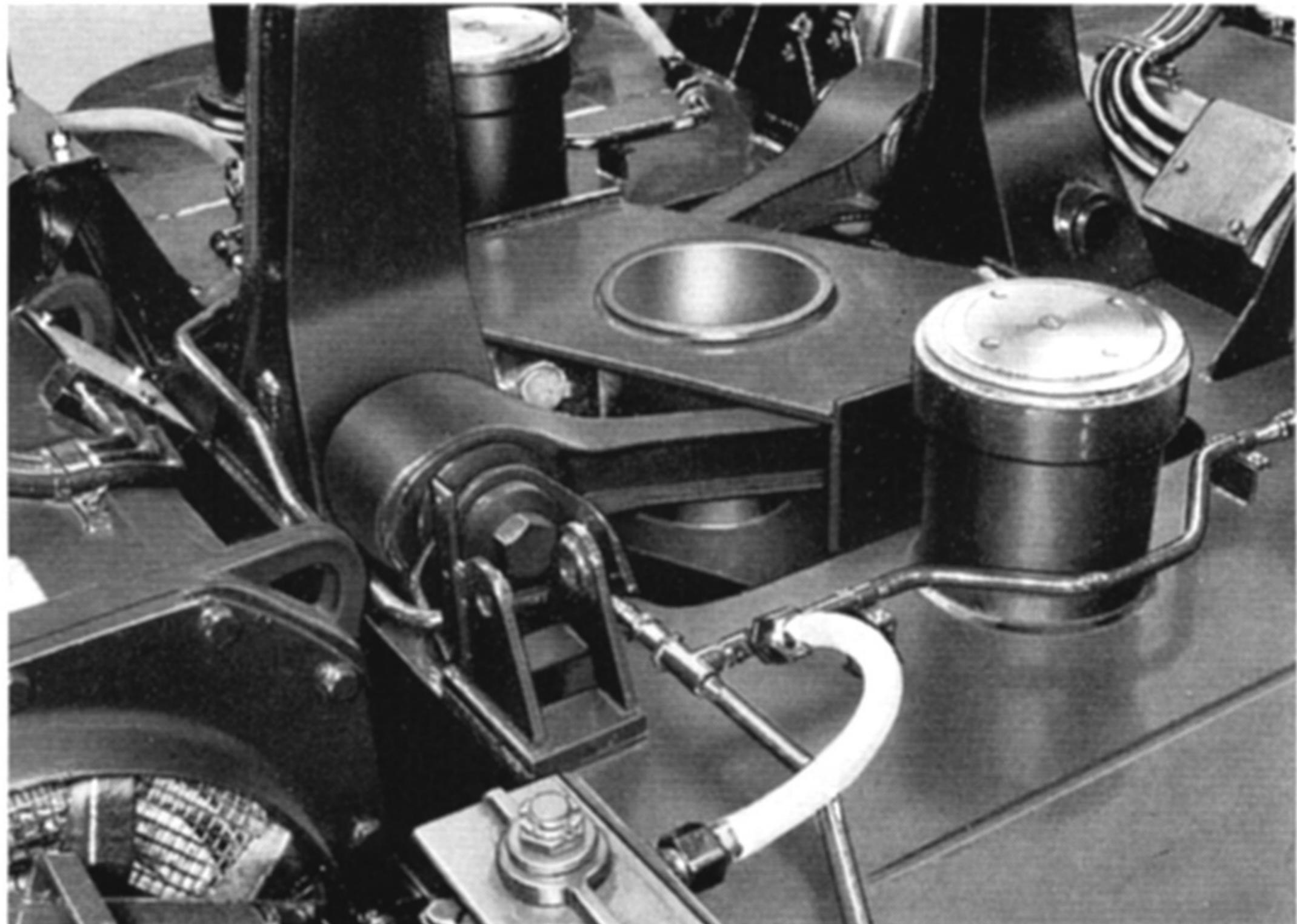
*The bogie pivot, free of vertical forces, transmits the acceleration and braking forces via a pair of links.*
